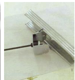
Failure mode: Breakage of profile guides.
