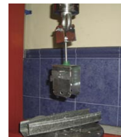
Sample subjected to load of 450 kg. Breakage of the profile
