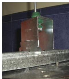
Sample subjected to load of 50 kg.
