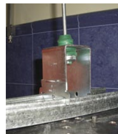
Sample subjected to load of 250 kg.
