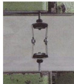
Sample subjected to load of 300 kg.
