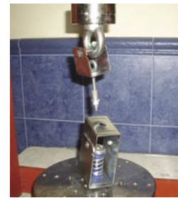
Detail of the sample subjected to load of 200 kg. Upper part breaks.
