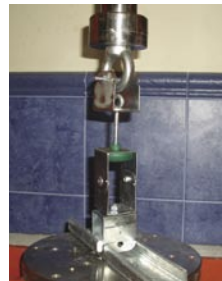
Sample subjected to load of 150 Kg.
