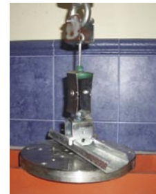
Sample subjected to load of 350 Kg.
