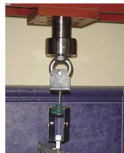
Sample subjected to load of 160 Kg.
