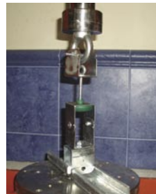
Sample subjected to load of 150 Kg.
