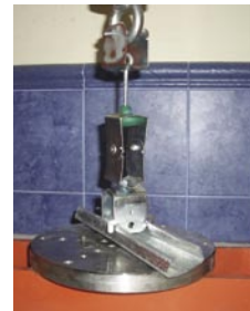
Sample subjected to load of 350 Kg.
