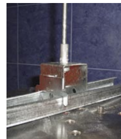
Sample subjected to load of 150 kg.
