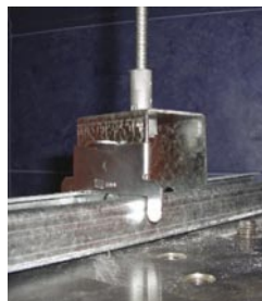
Sample subjected to load of 50 kg.
