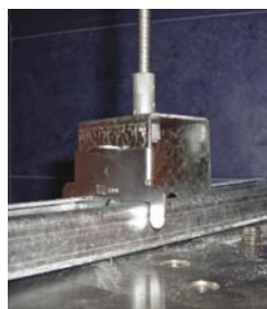
Sample subjected to load of 50 kg.
