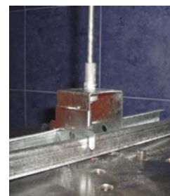
Sample subjected to load of 150 kg.
