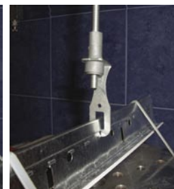
Sample subjected to load of 75 Kg.
