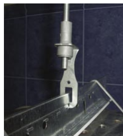
Sample subjected to load of 25 Kg.
